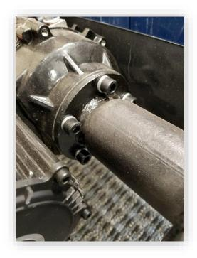
The final step is to remove either side axle assembly. When either axle is removed, the remaining axle that is still connected to the motor will have room to be able to drop away from the frame. Both axles are secured by five 6mm hex (Allen wrench) bolts. Ensure the motor to axle seal is salvaged is just the axle or motor is being replaced.
