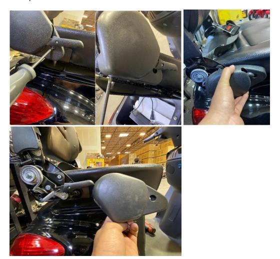
Lifting the seat up may make it easier to get to the screw on the bottom side. You will slide this plastic cover off the lever on the seat as shown in the photo.
