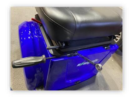
The seat is securing by two bolts, and the seat latch. The seat bolts are a 5mm hex head bolt on the bolt side, and 10mm on the nut side. Avoid overtightening or the seat will not be able to be lifted easily.
