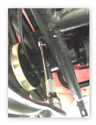
There are two transaxles to swing arm bolts on each side of the scooter. The bolt side is a Correct Size To Use. Make sure the bolts are tight on each side. If there is a gap between the axle bracket and the swing arm, this is normal. If overtightened bolts from the transaxle to swing arms can potentially snap.
