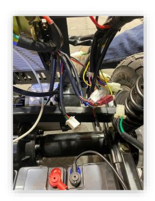
Once all connections have been replaced, remove the old wire harness and the entirety its mounts. Zip tie the new harness to the frame at the same points the old harness was mounted. Test that all functions of the scooter are working as they should prior to reinstalling the body paneling.
