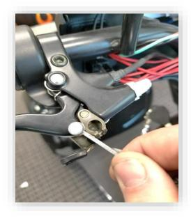
**Left Brake Handle Replacement** - To replace the left brake handle, start by removing the headlight shroud. Once removed, take of the securing nut and bolt. Both the nut and the bolt are 10MM.
