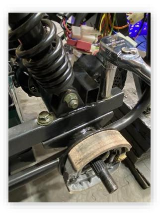
Once the rear wheels are removed, the next step is to remove the four 10mm axle to swing arm bolts. These bolts secure the transaxle assembly to the swing arms.
