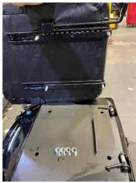
**Step Three** – Remove all 4 bolts using a *13mm* socket with a rachet. Be careful as there are 4 spacers as well that will be
