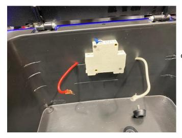
Your going to want to remove both wires going to the circuit breaker before removing the storage box.
