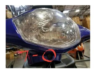
**Key Note** • The speedometer can be removed as well if needed once this has been completed. A 10mm soket and rachet can also be used to remove the outside bolt.
