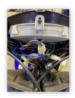
**Throttle Replacement** –To replace the throttle, start by removing the headset shroud. Once removed, separate the original throttle's electrical connector, and loosen (but do not remove) the 3 MM set screw for the original throttle. Disconnect both connectors and your job is complete.
