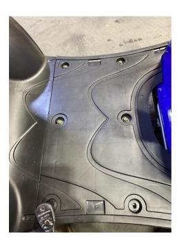
Remove the bolts on the back of the floorboard on the left and right side. Its going to be a Philips screw with a bolt that you must hold on to, to be removed. Be careful there are washers on the main body that need to be saved.
