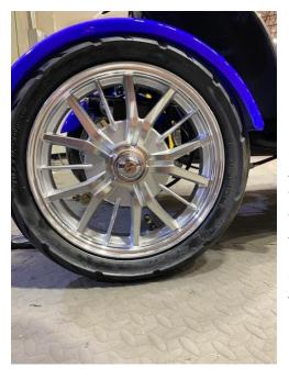
A jack or stand will be needed to remove the front tire. The front wheel is secured by the front axle bolt. On the wheel nuts there will be covers that need to just be popped off. The size your going to need is going to be a 19mm socket to take this off.
