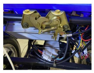
Remove the cable that goes to the truck lock. Your going to want to pull up in the meal/plastic part and remove the end of the cable. You're going to want to remove these the bolts along the running boards on both sides and in the middle.
