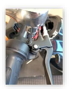
Right (Front)Brake Handle Replacement – To replace the right brake handle, start by removing the headlight shroud. Once removed, separate the brake handle's electrical connector. Once separated, remove any tension from the brake line by taking off the adjustment nut on the opposite end of the brake cable. Then, remove the cable from the brake handle as demonstrated in the photos below.
