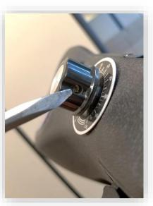
**Button Replacement** – To replace the high/low beam, turn signal, forward/reverse, or horn button, start by removing the headlight shroud. Once removed, locate the button you intend to replace, and separate the electrical connector. Then, dismount the original button by depressing the push clamps on each side of the button. A flat head screwdriver can help to depress the push tabs easier.
