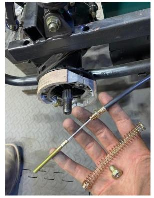
You will be using a 19mm wrench and a 6mm allen wrench to loosen the nut to take the axle bolt off.
